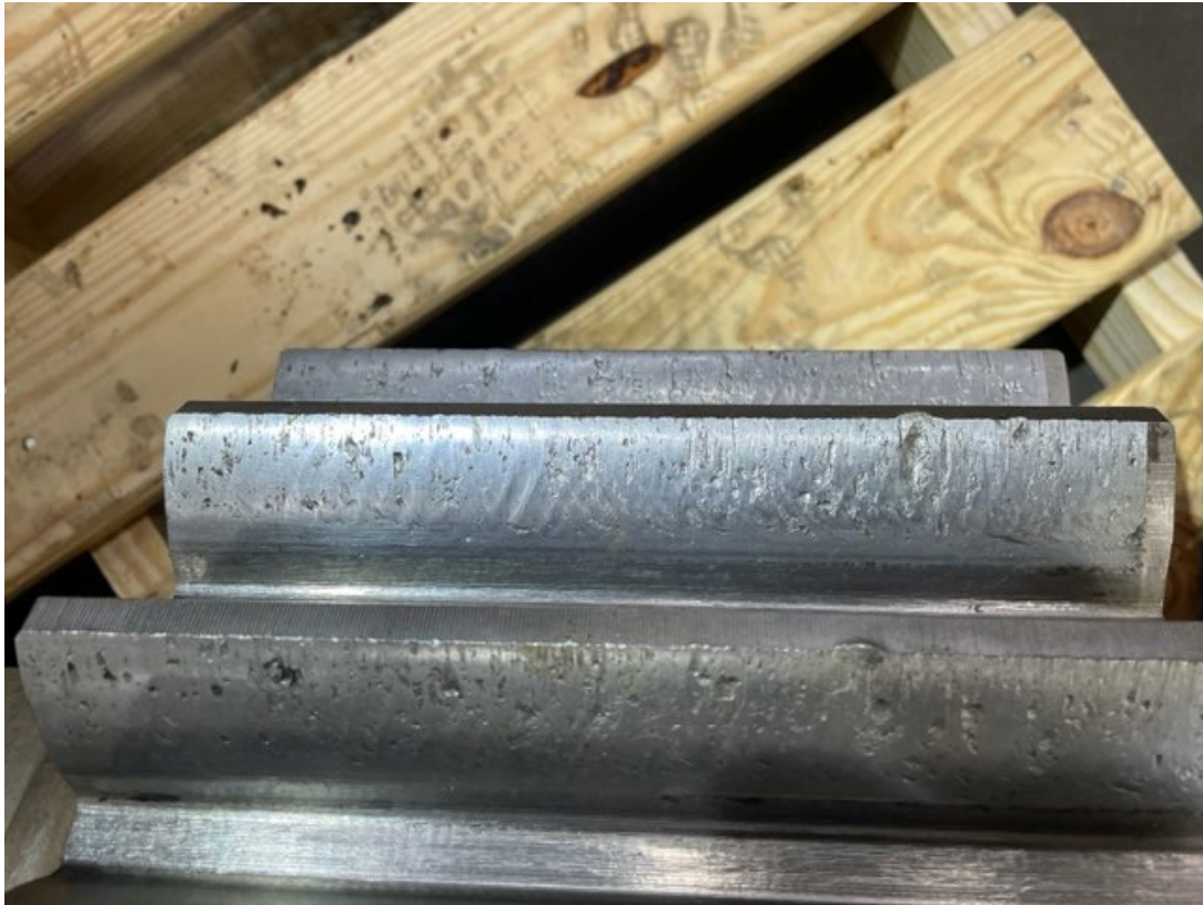
Pitting on south pinion gear
