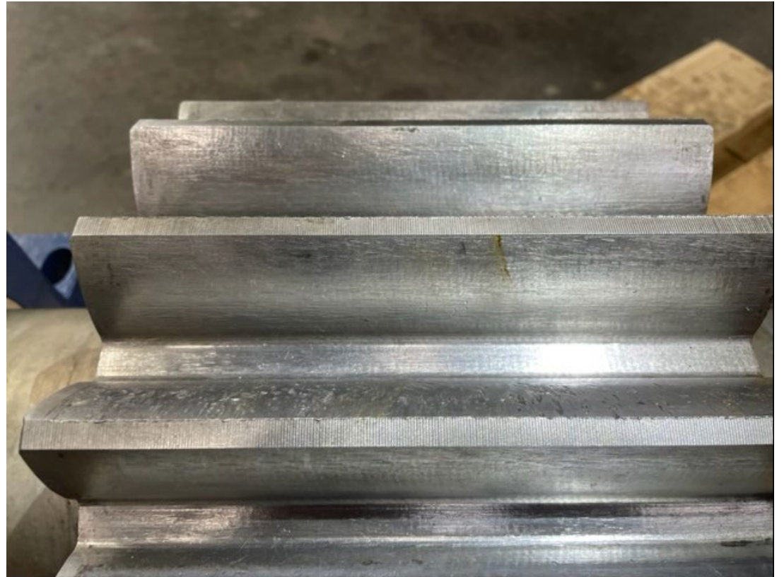
Unworn pinion gear
