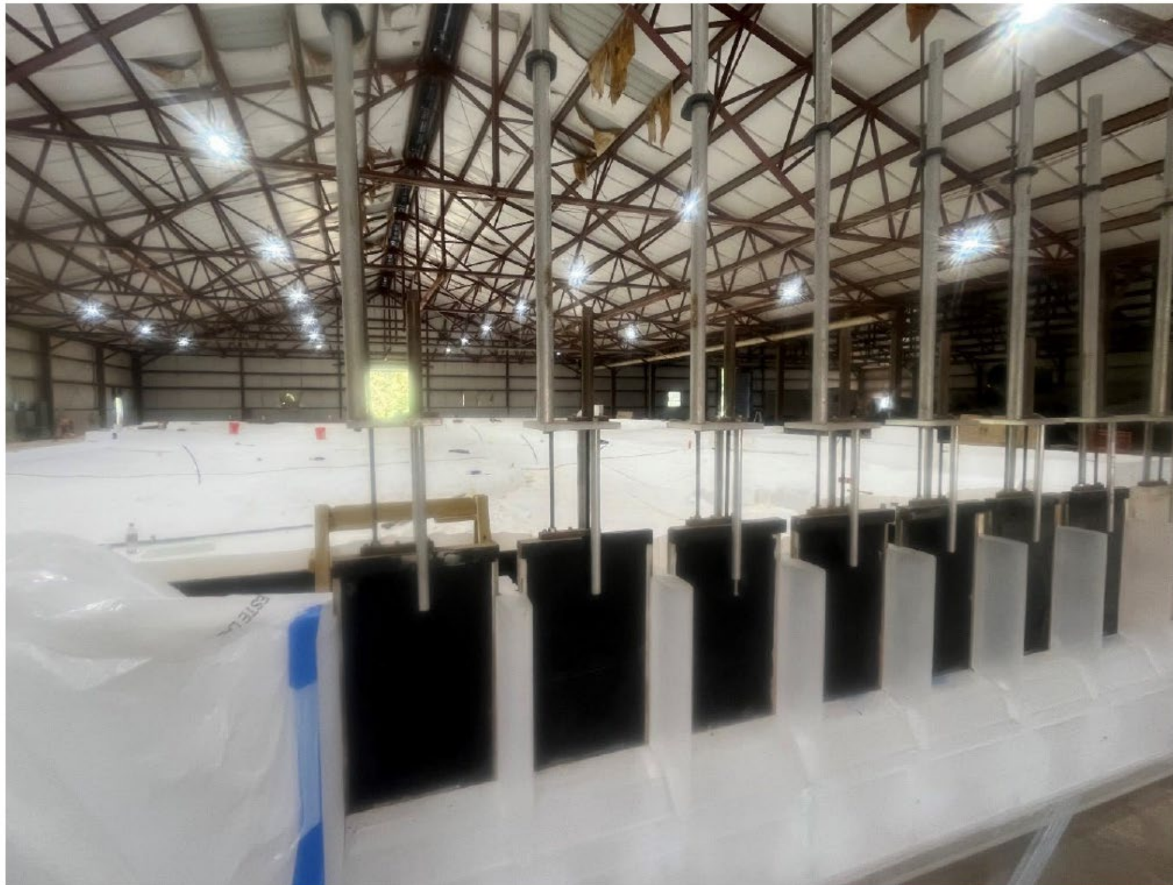
Figure 3. Repurposed gates from original McNary physical model.
